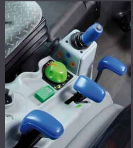
■ For higher performance and enhanced operator comfort, RF-RS-RV can also be equipped with an electronic rear hitch, electrohydraulic controls for the main engagement functions and a joystick lever for auxiliary control valves.
