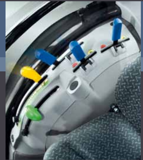
■ The control valves and mechanical hitch control are located on the side console.
